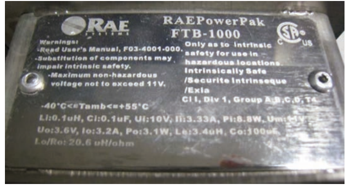
Figure 4: RAE Systems PowerPak U.S. and Canada hazardous-area certification label with clearly marked entity parameters.
