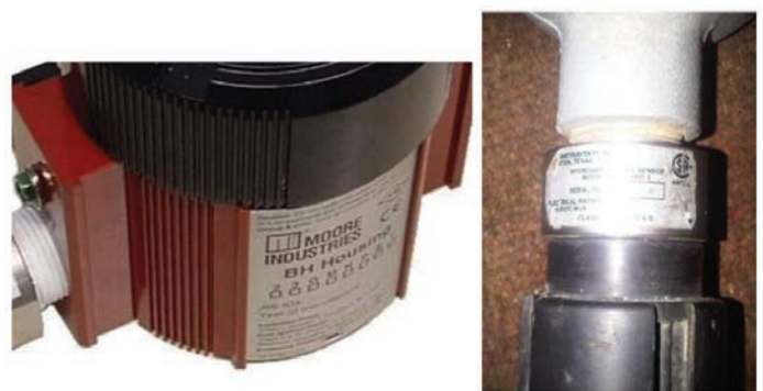
Figure 3: Component certification of housing and component certification of sensor module. Note that there is no equipment-level certification that includes both of these components.
