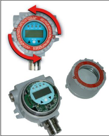
1. Unscrew the housing lid from the housing body by rotating it counter-clockwise. As shipped, one of the conduit holes is covered by the provided hex-head plug. The other conduit is shipped with connected wires.
