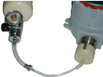
**RAEGuard LEL connected to gas cylinder with a calibration adapter.**
