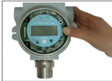
2. Tilt the retaining clip toward the housing to release the instrument assembly.
