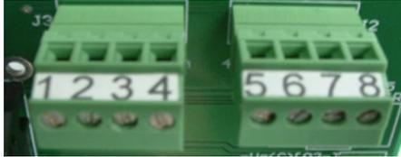
2. Lace the wires through the RAEGuard LEL's wire hole and connect wires to the corresponding pin numbers of the terminal blocks:
