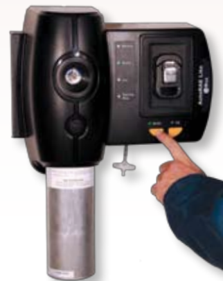
Bump testing ToxiRAE 3 with AutoRAE Lite Bump Test and Calibration Station
