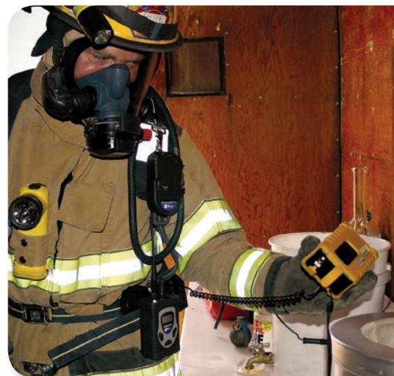
Hazardous Material Response Team member using MultiRAE Plus and GammaRAE II R with RAELink3
