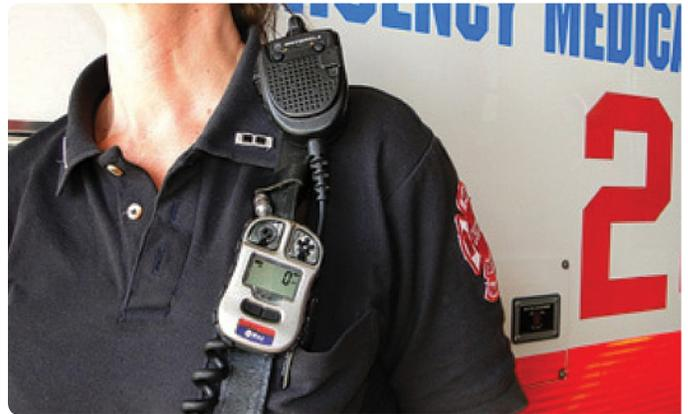
The Chicago Fire Department implemented new standards May 1 requiring paramedics to wear a small detector on their radio straps that alarm and provide readings on levels of carbon monoxide, a dangerous gas that accounts for thousands of deaths nationally each year.
