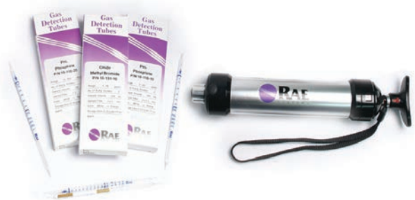
Figure 2. Gas detection tubes for MeBr and PH 3 with hand pump.
